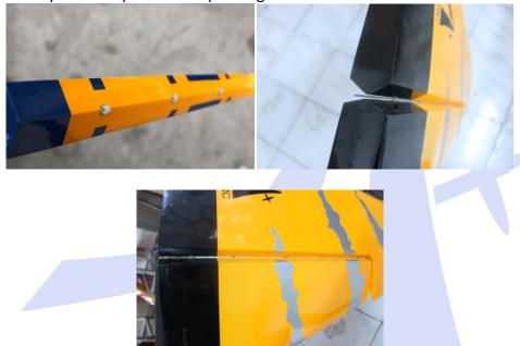
5. Glue the rudder horns in the rudder with epoxy; wipe off excess glue while it is wet.
