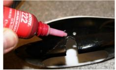
4. Fit the wheel pants over the wheel assemble and secure with 2 x cap head bolts.
