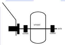
Note: Do not tighten up the collets yet as the wheel needs to be fitted so there is an equal distance within the wheel pant.
