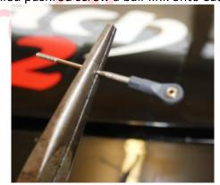
g. Using the supplied bolts attach the pushrod at both ends. Check to see you have sufficient movement of the aileron. If not adjust.
