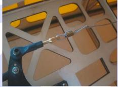
c. Crimp the cable using a pair of plies then trim cable.
