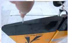
6. Glue in tiller mount and tighten tiller rod.
