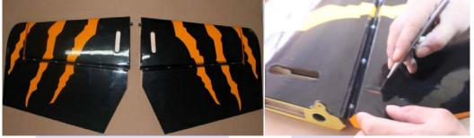
b. Before gluing the area on the horns that goes inside the elevator needs to be roughed up with sandpaper. This allows a better glue joint.
