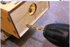
3. Mount the engine with the stand offs to the bulkhead. Remember to use large washers on the inside to spread the load and use plenty of thread-lock.
