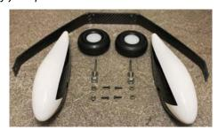
1. First Push each axle through the large holes and tighten up using 2 wrenches 13mm
