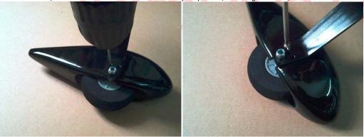
• Now line up the wheel in the centre of the wheel pant opening and tighten the collets. Remember to use nutlock and to make sure the wheel can move freely.
