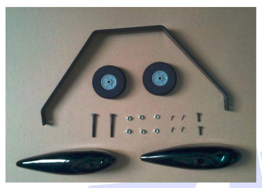
• Push each axle through the whell holes, and tighten up with 1x self locking nut and 1x blind nut. Then axle though the hole of landing gear, and tighten up with 1x self locking nut
