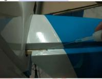
Remove the covering for the elevator servo
