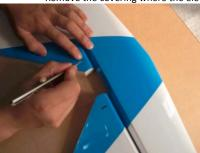
• The area on the horns that goes inside the elevator needs to be roughed up with sandpaper. This allows a better glue joint.
