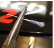
• Using supplied bolts attach the pushrod at both ends. Check to see you have sufficient movement of the aileron. If not adjust.
