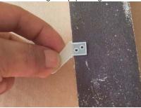
• Glue both horns in with epoxy glue, use a bolt through the horns when gluing to make sure the alignment is correct.
