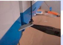
• Fit the arm onto the rudder servo and crimp the wires to a taut tension
