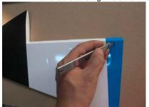
• Test fit the rudder horns
