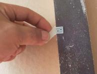
• Glue the rudder hinges into both the rudder and fin using CA. Remember to use vaseline on the hinge joint. While drying use tape to keep it in alignment.
