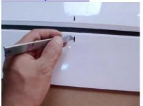
Using sand paper rough the area that will be glued into the aileron.
