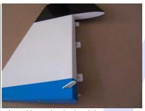
Sand the area on the horn that fits inside the rudder so the glue bonds better
