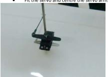
Using the pushrod supplied screw ball joints onto each end. The correct length will leave the aileron lined up to the inner part still attached to the wing.
