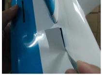
• Remove the covering where the elevator horns fit, use either a soldering iron or a sharp knife.
