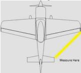
• Glueing – Once you think you are ready to glue, measure again. We recommend 2 methods for gluing. Either remove the covering on the area that is covered by the fuselage and glue with CA or leave the covering on and glue with thin cyno. Wicking in thin first, if a large gap is visible then use medium or thick. Remember to wick in small amounts at a time keeping the plane level, this will ensure the glue stays where it needs to be.
