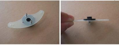
• Fit the rudder servo and drill holes using a fine drill for the servo screws, drop thin cyno into the holes to strengthen the wood.
