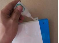
Glue the rudder horns through the rudder with CA. Use the ball joint and bolt while gluing to maintain alignment.
