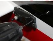
• Re-fit the elevator servo and secure it in with servo screws.
