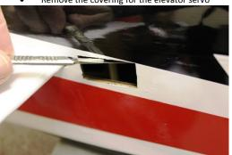
Remove the covering where the elevator horns fit, use either a soldering iron or a sharp knife.
