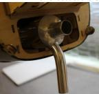
Cut out the area for the engine cylinder head and the exhaust outlet on a piece of thin card and tape this to the fuselage at one end.
