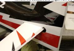
It is important that care is taken when aligning the rear stab. Measure each side to make sure that an equal amount shows on each side.
