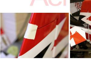
• Glue the rudder horns through the rudder with epoxy, wipe off excess glue while it is wet. Use the ball joint and bolt while gluing to maintain alignment. While still movable measure that the same amount pushes out each side. Care needs to be taken here otherwise your rudder geometry will be incorrect.
