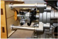
Exhaust options. Depending on the engine many exhaust options are available. Standard muffler, Pitts Exhaust of canister with header.
