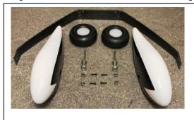
Push each axle through the large holes and tighten up using 2 spanners.
