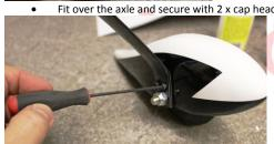
Now line up the wheel in the centre of the wheel pant opening and tighten the collets. Remember to use nutlock and to make sure the wheel can move freely.
