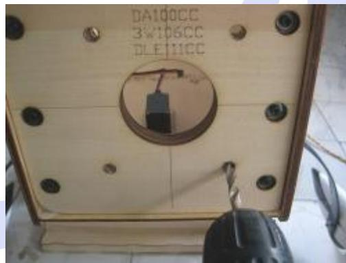
2. mount the engine with the stand offs to the bulkhead. Remember to use large washers on the inside to spread the load and use plenty of thread-lock.
