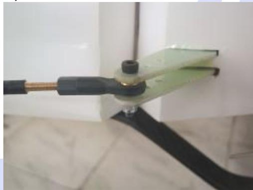
6. Installing the Rudder Servo
