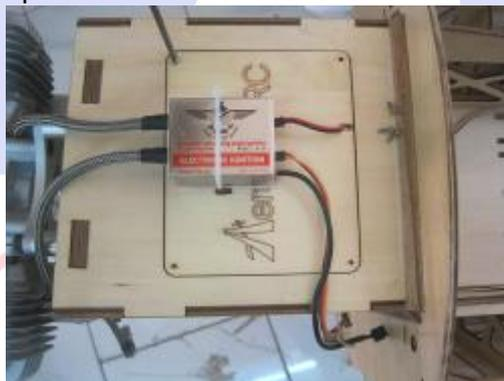
8. Mount the engines ignition to the motor box on radio foam to reduce vibrations.
