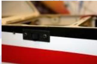
2. A convenient place to mount the RX is just in front of the rudder servo. Ensure that it is mounted on Velcro or radio foam and securely strapped down.
