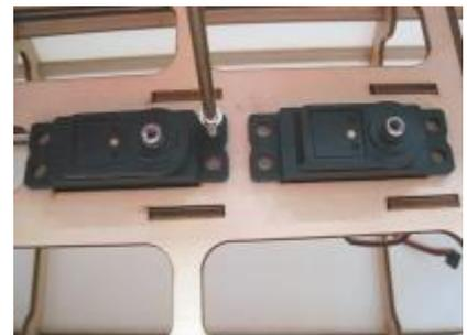
c. Using servo screws fix the servo in place, note the spline is towards the front of the plane.
