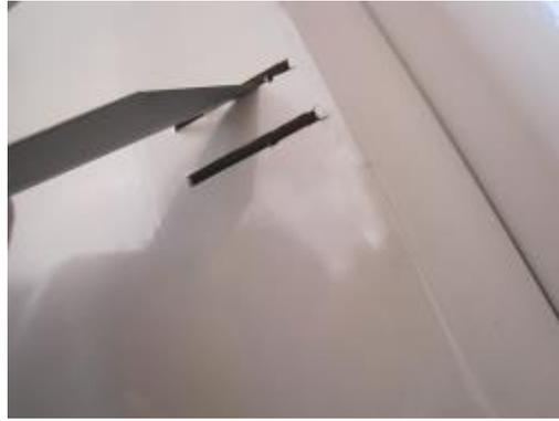
b. Using sand paper rough the area that will be glued into the aileron.
