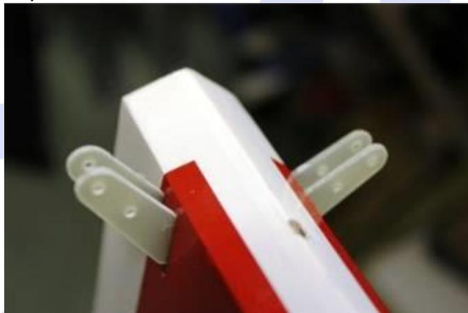
3. Sand the area on the horn that fits inside the rudder so the glue bonds better.
