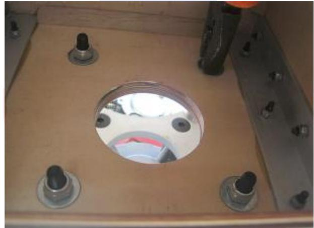
3. Exhaust options. The plane is equipped with a pipe tunnel so it will accommodate many kinds of exhaust including stock, cans, and pipes.
