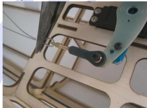
c. Crimp the cable using a pair of pliers then trim cable.
