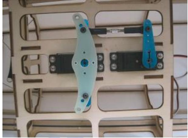
7. Installing the rudder cables
